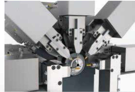
■ Bilateral milling mode Both 1 and 5 knife racks can be installed with one side power.
