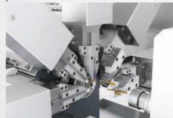
■ Back spindle The back side is a type 12 spindle,using the spindle end drill processing.
