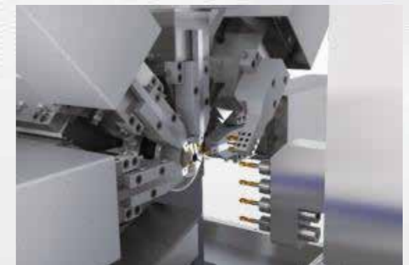
■ Multi-axis drilling on the back Back 4 ER11 spindle end
